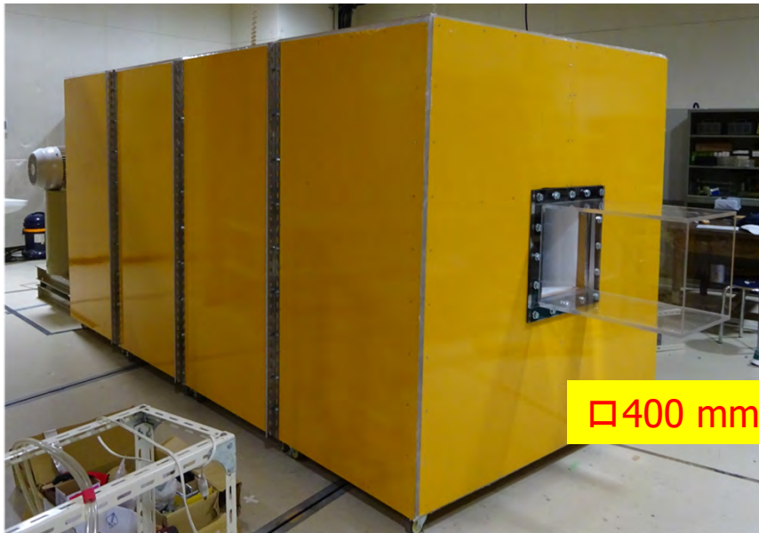
Fig. Experimental setup of the wind tunnel experiment
